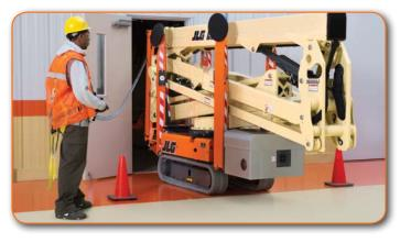
You also get the advantage of a first-to-market environmentally-friendly power system on these machines — they are outfitted with an optional breakthrough Lithium-lon electrical system that produces zero emissions and longer runtime, so the compact crawler boom runs clean while staying green.
